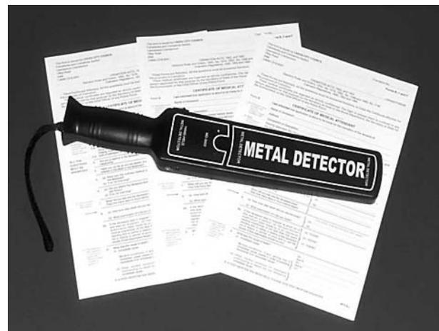
**Figure 1** The MD3003 hand held metal detector. The device is swept over the body after it has been placed on a non-metallic surface.
