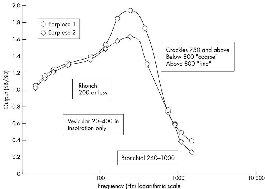
**Figure 2** Performance of the stethoscope bell and stethoscope diaphragm as measured at both earpieces. The crossover point is about 400 Hz (the differences in plots derived from the two earpieces may indicate that the microphone and preamplifier combination serving one were relatively less sensitive at higher frequencies than that serving the other).
