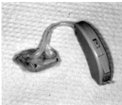
Figure 3 Behind-the-ear aid showing the earmold and plastic case.
